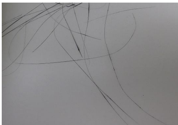
Figure 6.18 Fiber Spinning Using Lignin from 0% GL Extraction Experiment
