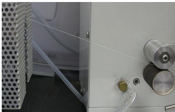
Figure 6.17 Linear Low-density Polyethylene (LLDPE) Fiber Spinning
