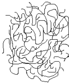
Figure 6.2 Completely Amorphous Polymers Exhibits Only a T_g Value ( http://faculty.uscupstate.edu/llever/Polymer%20Resources )
