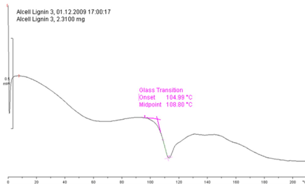
Figure 6.16 Typical Thermogram for Alcell Lignin (108.8°C)
